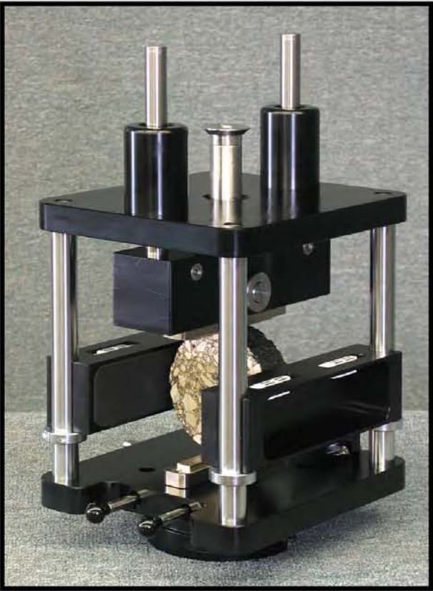
IDT Testing Fixture with Extensometer Guards in test position
