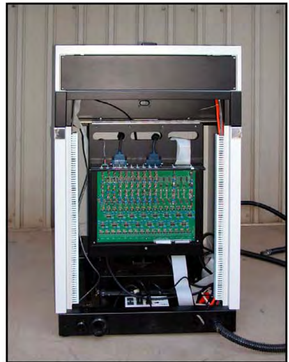
Operating Position rear access panel removed
